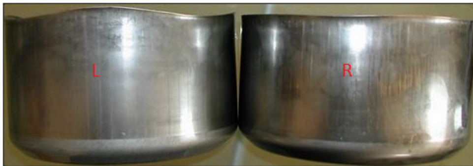
Figure 1: Different ear formation at room temperature formed from 1.4571 (L) & 1.4539 (R).
